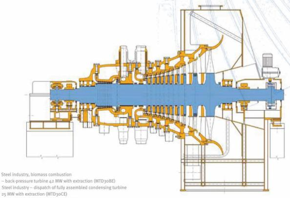
3 Cross section of condensing turbine with reheating (MTD4oCR)
