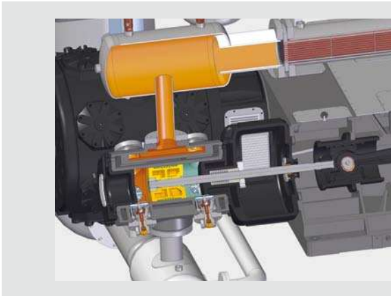
COOLING BETWEEN STAGES
